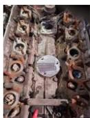
If you have bought the waste spark system, you must remove the distributor and replace it with the included coil bracket. You can use the original distributor screws and O-ring. Mount the two coils with the connectors placed at the lower half of the coils.
