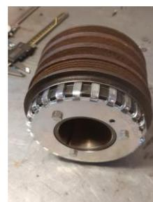
Remove the crank pulley with its damper, if you have a Marelli or later engine you remove the original triggerwheel and mount the new one with the included shim ring and you can use the old screws, the triggerwheel is located correct by one dowel. If you have a pre Marelli engine you need to get a Marelli type crank pulley (harmonic damper) to do this.
