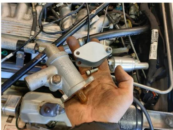
Open the radiator cap (on the expansion tank) to depressurise the coolant system. Remove the AAV valve at the rear left corner of the engine, install the included blanking plate with the original screws.
