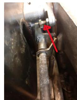
When doing this it is important to turn the main center top disc by holding the aluminium disc itself and not put your fingers on the rod ends. This is because you want to adjust the rods to take up the slack in the rod ends of the disc also. You will not do that if you put your fingers on the rodends.
