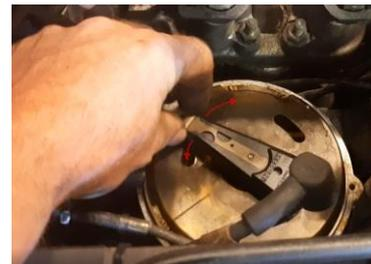
Take off the rotor and drip some oil into the shaft centre. If everything is free to move it is fine, if not, you need to overhaul your distributor, buy a new one or consider the waste spark system. When this is ok mount the rotor and cap again. Take off the vacuum line to the distributor and blank off the rubber hose (to avoid false air getting in). Start the engine and check the ignition setting with a lamp and looking on the front pulley and its degree wheel.
