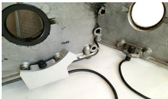
If you have a Marelli or later engine the new crank sensor should fit on the original trigger sensor bracket. (Right in the picture)
